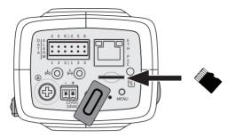
Figure 5.7 Inserting an microSD card
